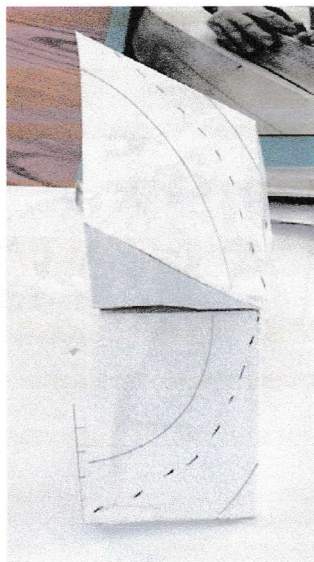
Folded drawing: drawing for ascending volute folding into oblique plane for handrail to lie on
