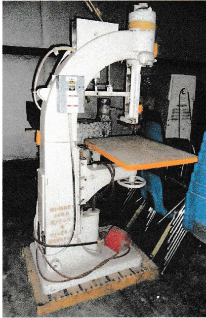
Wysong & Miles Co. drill press— has been converted to air feed, used for 1 operation, bought the machine cheap enough to dedicate in such a way, $75 in 2004.
